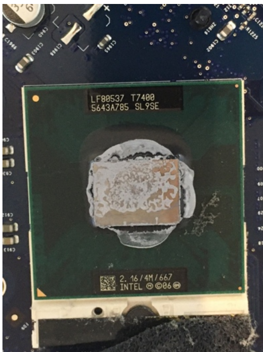
Figure 21 - iMac Intel Core2Duo CPU before cleaning
