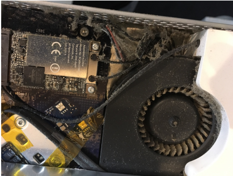
Figure 20 - The cooling system blocked with dust.
