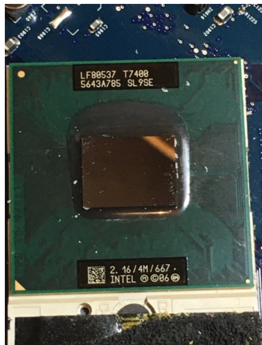
Figure 22 - iMac Intel Core2Duo CPU after cleaning
