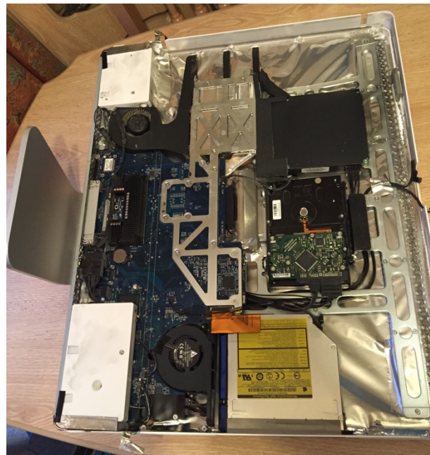
Figure 1 - Inside a 24" iMac Core2Duo
