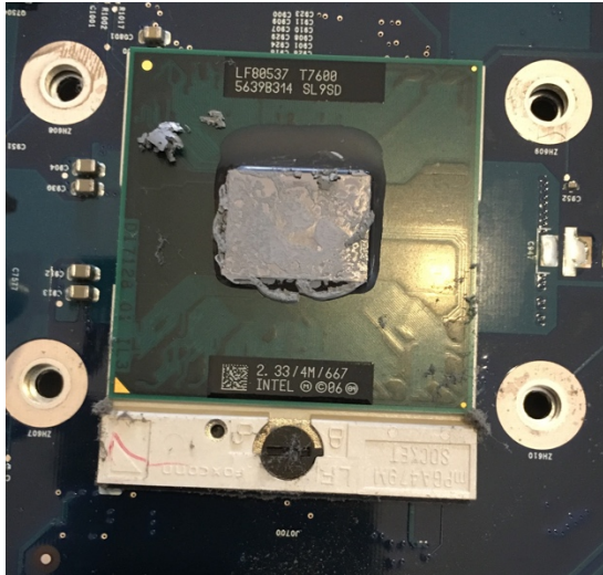
Figure 7 - iMac CPU with dried thermal paste
